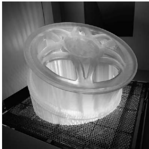
A part produced by Stereolithography
